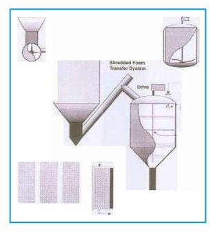
Foam pieces from various sources - production trim and post-consumer waste - can be suitable for rebonding, although in practice production trim and cuttings are by far the most commonly processed. Granulators and flock-mills are normally used to shred the foam into pieces approximately one centimeter in diameter. There are other technologies available to handle large foam pieces by cutting them into very thin strips, which can then be reduced into smaller pieces.
